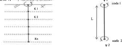
Discrete element model for torsional response of Pile (Chow, 1985) 桩扭转响应的离散元模型
